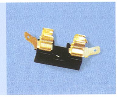
Explanaion of specification: suitable fuse 05.25x20mm Maximum rated value: 6A 250V AC Holder: Flame-rated value: 6A 250V AC Holder: Flame-retard plastic Clip pole: Silver- plating brass
