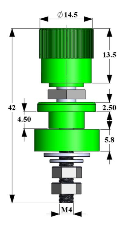
Binding Post Insulated Standard With Thumb Nut-Grounded Type
