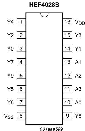
Fig 3. Pin configuration
